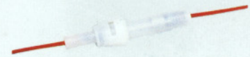
FC-F-0490 (SY021) Suitable fuse: \phi 6 \times 30 \text{MM} Greatest specified value: 6 \text{A}, 250 \text{V.AC} Able to bear the high temperature: 80^\circ \text{C} Material: (PE) Polythene
