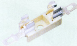
FC-F-0501 (SY034) Suitable fuse: \phi 5 \times 20 \text{MM} Greatest specified value: 6A.250V.AC Base of the seat: Fire Resistant High Temperature Standing Plastic
