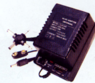
FC-F-0069 (LLA1000) LLA1000-Plug-in adapter Input voltage: 110V or 220V or 110/220V AC Selectable output voltage: 1.5/3.0/4.5/6.0/7.5/9.0/12 V DC Maximum load: 1000mA Input plug: AT ET SAA ST VDE Output plug: 6 way universal connector
