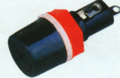
FC-F-0487 (SY015) Suitable fuse: \phi 5 \times 20 \text{MM} Exposed to resistance: < 0.02 \Omega Able to bear pressing: \geq \text{AC}3000 \text{V} Insulating resistance: \geq 1000 \text{M}\Omega Material: Bakelite
