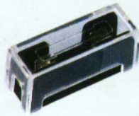
FC-F-0500 (SY033) Suitable fuse: \phi 5 \times 20 \text{MM} Greatest specified value: 6A.250V.AC Base of the seat: Fire Resistant High Temperature Standing Plastic
