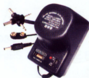
FC-F-0073 (LLA500G/LLA300G) LLA500G(LLA300G)-Plug-in adapter Input voltage: 110V or 220V or 110/220V AC Selectable output voltage: 1.5/3.0/4.5/6.0/7.5/9.0/12 V DC Maximum load: 500mA(300mA) Input plug: AT ET SAA UK RUK Output plug: 6 way universal connector
