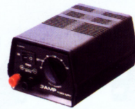
FC-F-0071 (LLA3000) LLA3000-Desk top adapter Input voltage: 110V 60Hz or 220V 50Hz or 110/220V 60/50Hz Selectable output voltage: 3.0/4.5/6.0/7.5/9.0/12 V DC Maximum load: 3000mA Input plug: AT BS SAA
