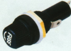
FC-F-0483 (SY004) Suitable fuse: \phi 6 \times 30 \text{MM} Exposed to resistance: < 0.02 \Omega Able to bear pressing: \geq \text{AC}3000 \text{V} Insulating resistance: \geq 1000 \text{M}\Omega Material: Bakelite
