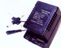
FC-F-0075 (LLA1000B) LLA1000B-Plug-in adapter Input voltage: 110V or 220V or 110/220V AC Selectable output voltage: 1.5/3.0/4.5/6.0/7.5/9.0/12 V DC Maximum load: 1000mA Input plug: AT ET SAA ST VDE Output plug: 4 way universal connector
