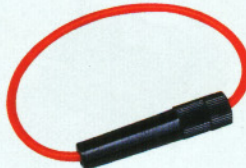
FC-F-0489 (SY020) Suitable fuse: \phi 6 \times 30 \text{MM} Able to bear pressing: \geq \text{AC}3000 \text{V} Insulating resistance: \geq 1000 \text{M}\Omega Material: Bakelite
