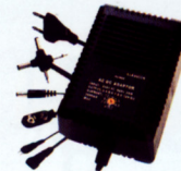
FC-F-0066 (LLA3000N) LLA3000N-Desk top adapter Input voltage: 110V or 220V or 110/220V AC Selectable output voltage: 3.0/4.5/6.0/7.5/9.0/12 V DC Maximum load: 3000mA Input plug: AT BS SAA Output plug: 6 way universal connector
