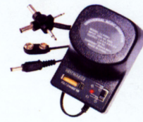
FC-F-0072 (LLA500J/LLA300J) LLA500J(LLA300J)-Plug-in adapter Input voltage: 110V or 220V or 110/220V AC Selectable output voltage: 1.5/3.0/4.5/6.0/7.5/9.0/12 V DC Maximum load: 500mA(300mA) Input plug: AT ET SAA ST Output plug: 6 way universal connector
