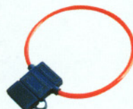
FC-F-0492 (SY023) Suitable fuse: \phi 6 \times 30 \text{MM} The outer cover is able to bear pressing: \text{AC}1000 \text{V} Able to bear the high temperature: 90^\circ \text{C} Material: ABS Polythene (ABS)
