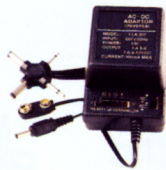
FC-F-0067 (LLA300) LLA300-Plug-in adapter Input voltage: 110V or 220V or 110/220V AC Selectable output voltage: 3.0/4.5/6.0/7.5/9.0/12 V DC Maximum load: 300mA Input plug: AT ET SAA ST VDE Output plug: 6 way universal connector
