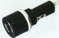
FC-F-0486 (SY014) Suitable fuse: \phi 6 \times 30 \text{MM} Exposed to resistance: < 0.02 \Omega Able to bear pressing: \geq \text{AC}3000 \text{V} Insulating resistance: \geq 1000 \text{M}\Omega Material: Bakelite
