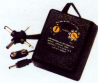
FC-F-0061 (LLA300N) LLA300N-Plug-in adapter Input voltage: 110V or 220V or 110/220V AC Selectable output voltage: 1.5/3.0/4.5/6.0/7.5/9.0/12 V DC Maximum load: 300mA Input plug: AT ET SAA ST UK Output plug: 6 way universal connector
