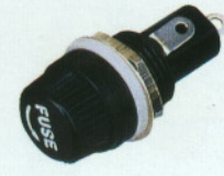
FC-F-0484 (SY005) Suitable fuse: \phi 5 \times 20 \text{MM} Exposed to resistance: < 0.02 \Omega Able to bear pressing: \geq \text{AC}3000 \text{V} Insulating resistance: \geq 1000 \text{M}\Omega Material: Bakelite
