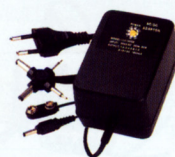
FC-F-0065 (LLA1500N) LLA1500N-Desk top adapter Input voltage: 110V or 220V or 110/220V AC Selectable output voltage: 1.5/3.0/4.5/6.0/7.5/9.0/12 V DC Maximum load: 1500mA Input plug: AT BS SAA Output plug: 6 way universal connector
