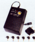
FC-F-0063 (LLA600N) LLA600N-Plug-in adapter Input voltage: 110V or 220V or 110/220V AC Selectable output voltage: 1.5/3.0/4.5/6.0/7.5/9.0/12 V DC Maximum load: 600mA Input plug: AT ET SAA Output plug: 6 way detachable plug
